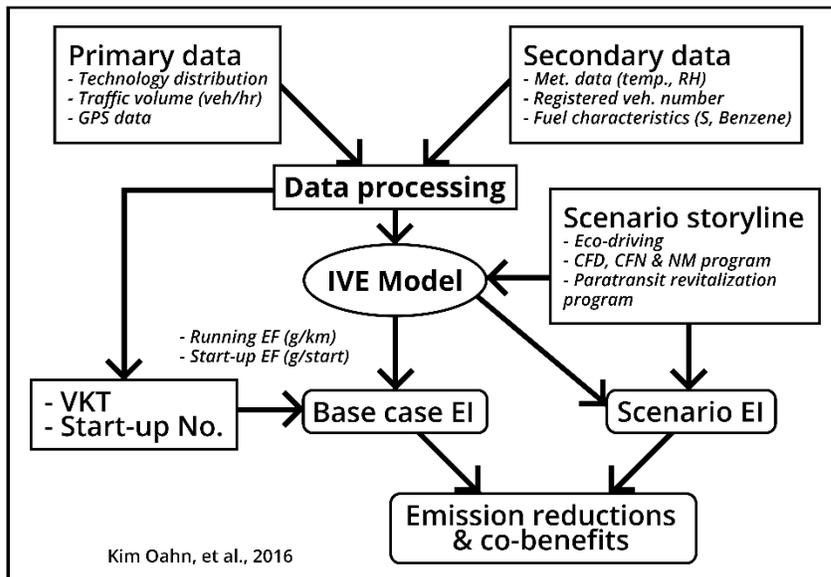
Shown in this figure is the overall design of an EI with modeling included. Focus on the aspect of data availability the collection. Under Primary and Secondary data that are collected, emissions will be calculated to arrive at a 'Base case EI'.
