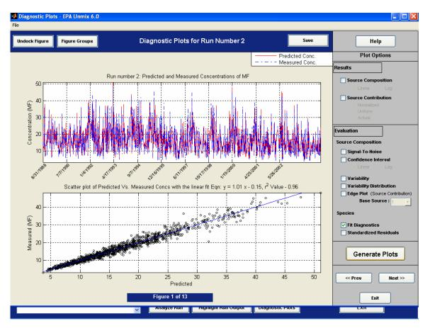
Figure 15: Diagnostic Plots – Fit Diagnostics Example
