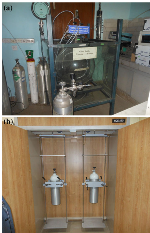
Fig. 3 Examples of gas preparation facilities for gas concentrations standards for: a a volumetric mixing chamber with clean gas dilution system (Indian Central Pollution Control Board, Delhi), and b a precise weighing system for quantifying gases compressed into a cylinder. The empty cylinder on the right has the same dimensions as the primary standard cylinder on the left and accounts for air displacement buoyancy effects (Indian National Physics Laboratory, New Delhi)
